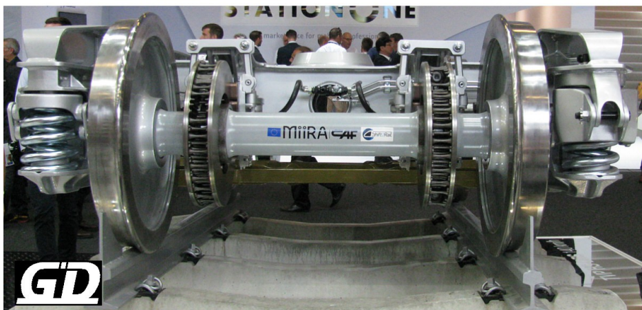
Güterwagen-Drehgestell TVP HS-DBS (High Speed - Disc Brake System) Freight Car Bogie TVP HS-DBS (High Speed - Disc Brake System)
