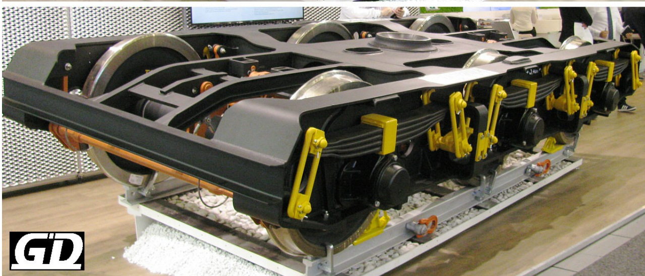
3-achsiges Güterwagen-Drehgestell Astra 3ASLs1o-K(V) 3-axle Freight Car Bogie Astra 3ASLs1o-K(V)
